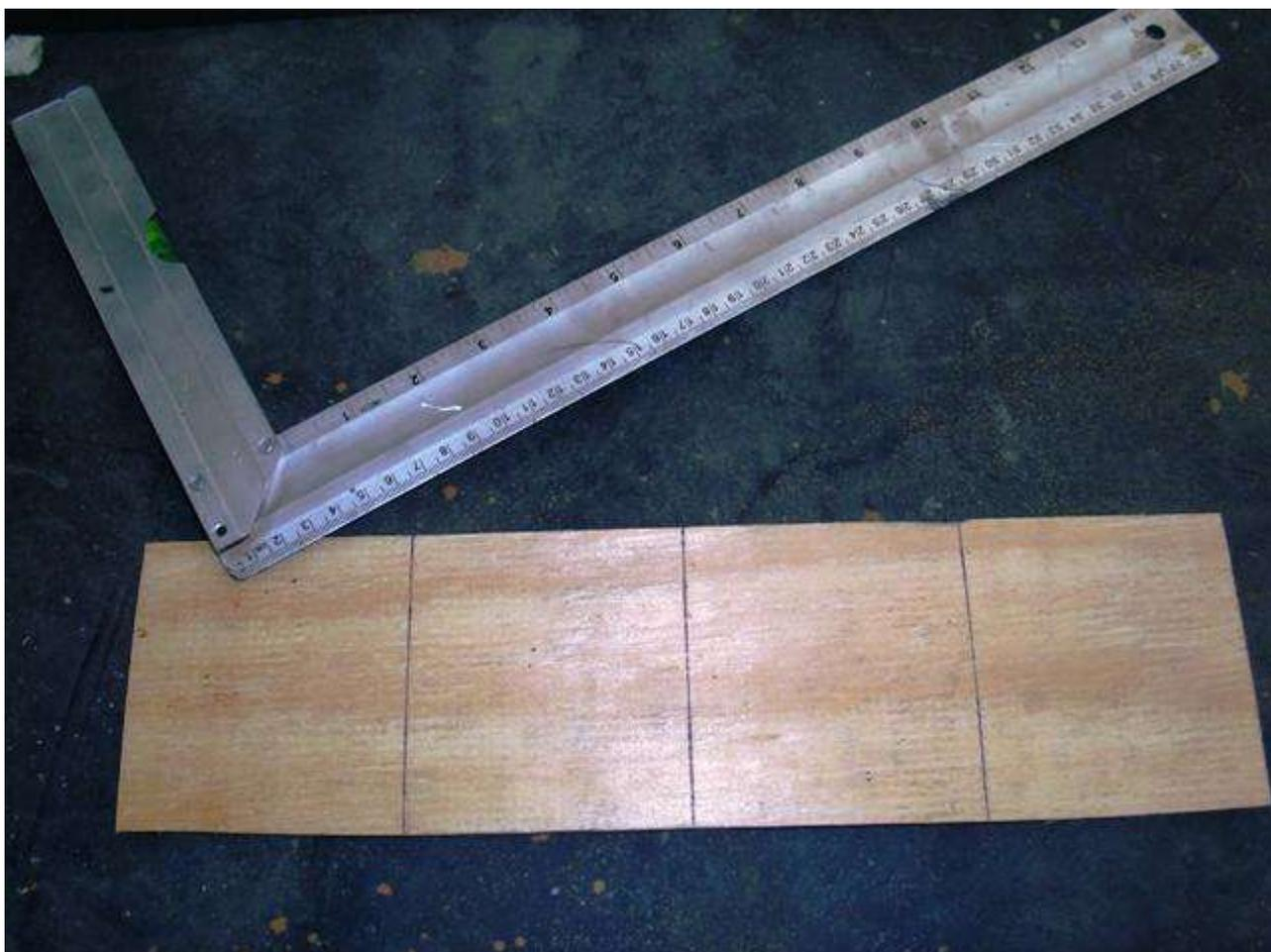
Using a saw place a small notch on the end of each line:
